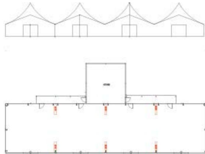
Blank floor plan showing individual pods and beam locations.
